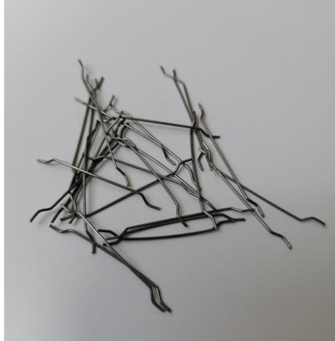
This kind of steel fiber is a high-performance steel fiber, which can improve the impact resistance and fatigue resistance of concrete; improve the impermeability of concrete. Because of its high tensile strength, good toughness, and low price, it is often used as a substitute for steel fiber.
